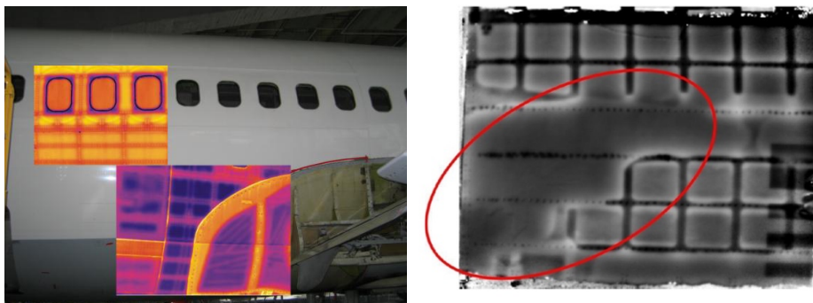
Figure. 11. C-Check IR active thermography system. Variants of execution and application.
