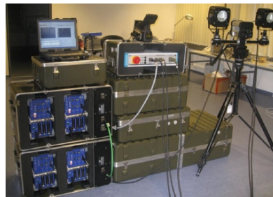
Figure. 11. C-Check IR active thermography system. Variants of execution and application.
