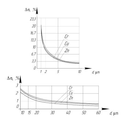
Figure 5. The maximum permissible deviation bases conductivity  $\sigma_b(d)$  of calibration standards
