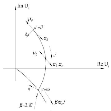
Figure 3. Functional connection insert voltage  $\mathring{U}_i$  from measurement value d and influence parameters  $\sigma_b, \mu_b, \sigma_c$
