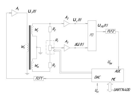
Figure 1. Block scheme of eddy current phase probe:
