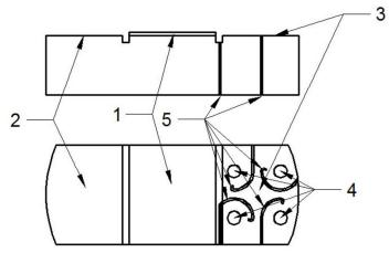
Figure 9. General view of calibration standard: 1 – area with metallic coating; 2 – area without coating; 3 – area measuring the conductivity of the base metal; 4 – contacts for connecting the cables of the power supply, ammeter and voltmeter; 5 – figured cuts
