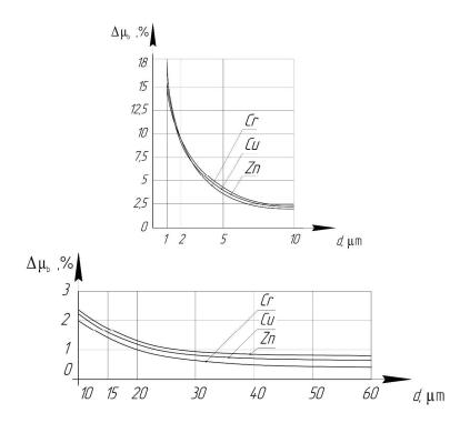
Figure 6. The maximum permissible deviation bases permeability  $\mu_b(d)$  of calibration standards
