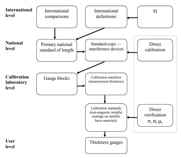
Figure 8. Four-level structure of the metrological chain to define and disseminate metallic coating thickness measurement scales
