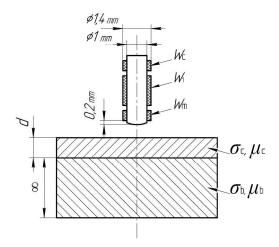
Figure 4. Model of the eddy current sensor of three-winding probe on the two-layer calibration standard
