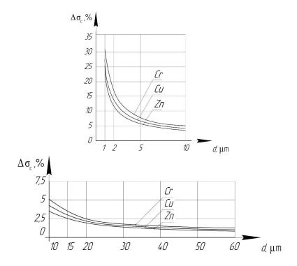
Figure 7. The maximum permissible deviation coating conductivity  $\sigma_c(d)$  of calibration standards
