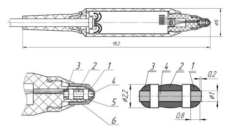
Figure 2. Consignment phase probe with a miniature sensor and removable protective cap: 1 - measuring  $W_{\rm m}$ , 2 - exciting  $W_{\rm 1}$  and 3 - compensating  $W_{\rm c}$  windings, 4 - ferrite core, 5 - cap 6 - housing
