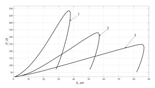
Figure 9. Load-displacement diagram curves for steel (1), brass (2) and aluminum (3) test blocks.
