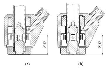
**Figure 4.** The position of the induction coil relative to the surface of test piece for standard (a) and modified (b) type D impact device.
