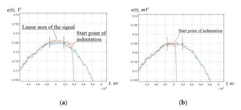
Figure 5. Signal obtained using a standardized (a) and modified (b) Leeb D impact device.
