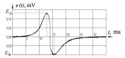
**Figure 2.** Graph of EMF e(t), induced in induction coil during measurement.
