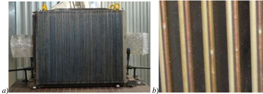
Figure 4. a) Surges on welds, b) close-up surges
